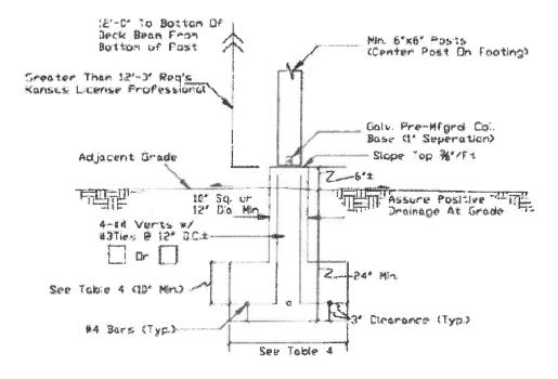
Note Footing May Be Incorporated Into Concrete Slab With A Minimum It Superation Between Bottom of Post And Slab
